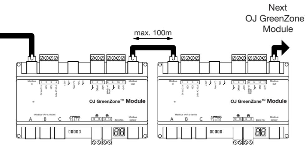
Fig. 5 - "Modbus in" connector
