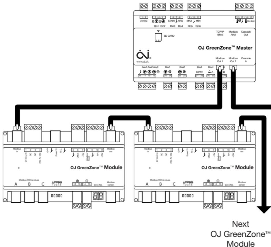
Max. 25 OJ GreenZone™ Modules M connected to each OJ GreenZone™ Master
