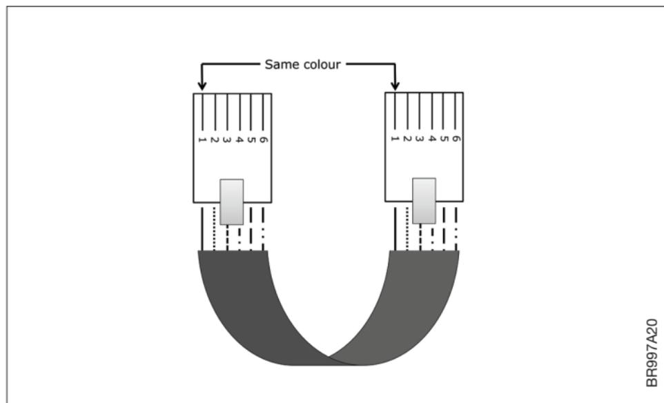
Fig. 7 - Connection of power supply voltage
